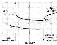
Peak load 50A (resistive) for 5ms Output voltage dips from 48V to 37V.
