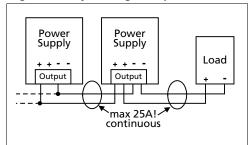
Fig. 12-2 Using distribution terminals
