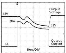
Peak load 20A (resistive) for 50ms Output voltage dips from 48V to 32V.
