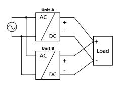
Energize all units at the same time to avoid the overload Hiccup<sup>PLUS</sup> mode. It also might be necessary to cycle the input power (turn-off for at least five seconds), if the output was in Hiccup<sup>PLUS</sup> mode due to overload or short circuits and the required output current is higher than the current of one unit.
