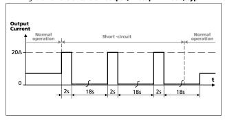
Fig. 6-4 Dynamic overcurrent capability, typ.
