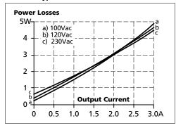
Fig. 8-4 Losses vs. input voltage at 5V, 3A, typ.
