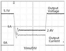
Peak load 6A (resistive load) for 50ms Output voltage dips from 5.1V to 2.4V.
