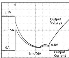
Peak load 15A (resistive load) for 5ms Output voltage dips from 5.1V to 0.8V.
