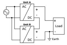
orientations other than the standard mounting orientation (input terminals on the bottom and output terminals on top of the unit). Pay attention that leakage current, EMI, inrush current, harmonics will increase when using multiple power supplies.
