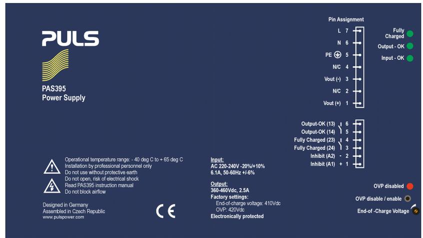
**Inhibit Input:** A signal voltage of at least 18V on the inhibit input terminal stops the charging mode. Safety features are not included. The input is galvanically isolated by an optocoupler. Typ. signal current; 4.2mA at 18V and 5.4mA at 24V.
