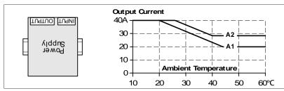
Fig. 25-12 Mounting Orientation C (Table-top mounting)
