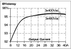
Fig. 11-3 Efficiency vs. input voltage at 24V, 40A, typ.
