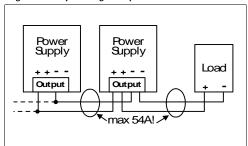
Fig. 14-2 Using distribution terminals
