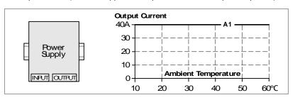
Fig. 25-11 Mounting Orientation B (Upside down)
