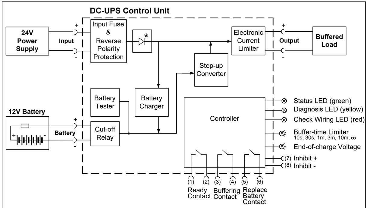
\*) Return current protection; This feature utilizes a MOSFET instead of a diode in order to minimize the voltage drop and power losses.
