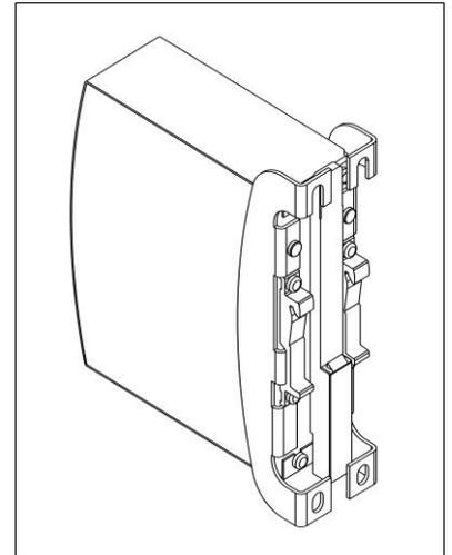
Fig. 23-8 Wall/panel mounting, side view
