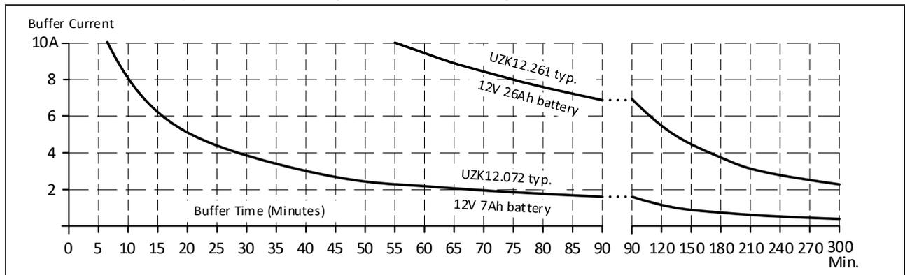
The battery capacity is usually specified in amp-hours (Ah) for a 20h discharging event. The battery discharge is non-linear (due to the battery chemistry). The higher the discharging current, the lower the appropriate battery capacity. The magnitude of the reduction depends on the discharging current as well as on the type of battery. High current battery types can have up to 50% longer buffer times compared to regular batteries when batteries will be discharged in less than 1 hour.
