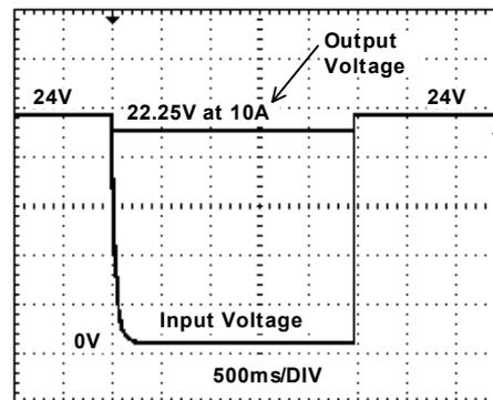
Fig. 5-4 Output voltage vs. output current in buffer mode, typ.
