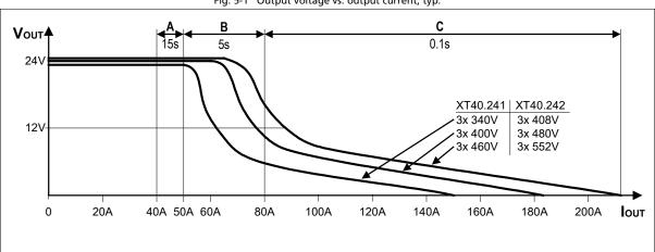
Fig. 5-1 Output voltage vs. output current, typ.
