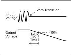
Fig. 6-2 Hold-up time vs. input voltage
