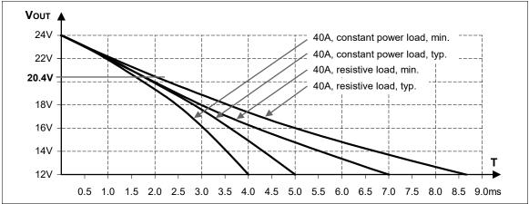
Note: At no load, the hold-up time can be up to one minute. The green DC-OK LED is on during this time.
