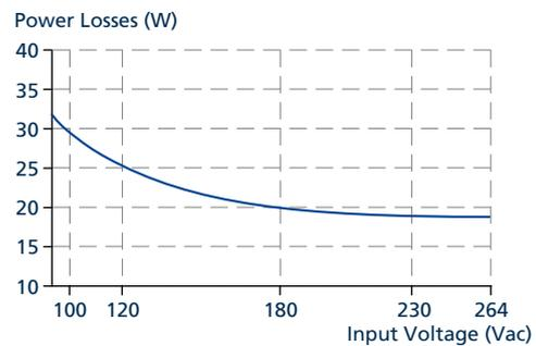
Fig. 9-4: Losses vs. input voltage at 48 V, 10 A, typ.
