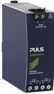
The YR40.482 is a dual redundancy module, which can be used to build 1+1 or N+1 redundant systems. The device is equipped with two 20A nominal input channels, which are individually decoupled by utilizing MOSFET technology. The output can be loaded with a nominal 40A continuous current.
