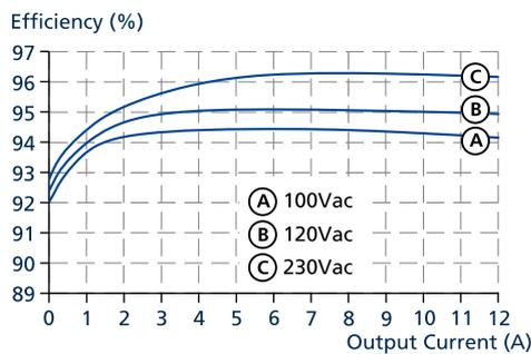
Fig. 9-1: Efficiency vs. output current at 48 V, typ.
