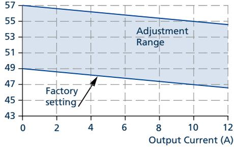
Fig. 6-4: Output voltage in "parallel use" mode, typ.
