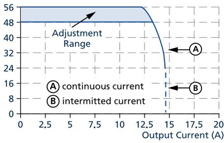
Fig. 6-1: Output voltage vs. output current, typ.
