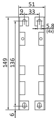
Fig. 23-5: Hole pattern for wall mounting
