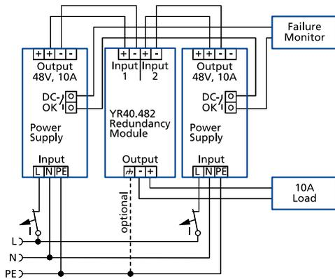
Fig. 24-5: 1+1 Redundant configuration for 10A load current with a dual redundancy module
