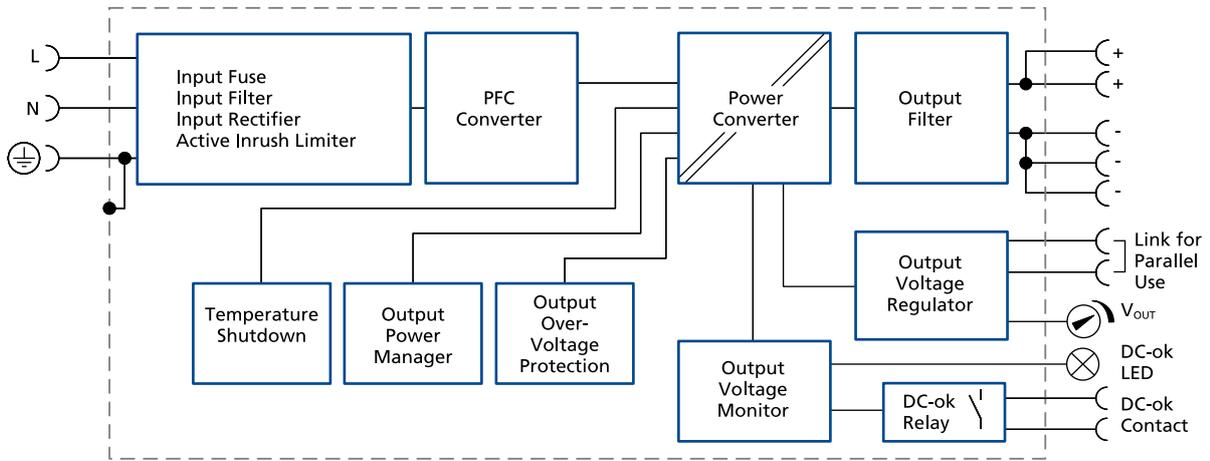
Fig. 12-1: Functional diagram
