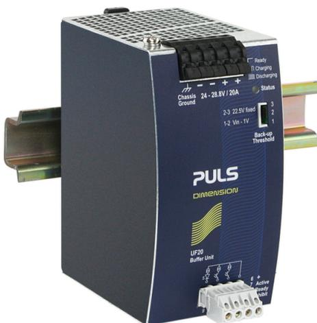
The UF20.481 buffer module is a supplementary device for DC 48V power supplies. It delivers power to bridge typical mains failures or extends the hold-up time after the AC power is turned off.
