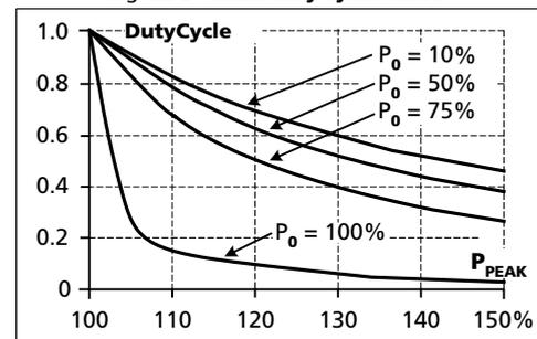
$$\text{DutyCycle} = \frac{T_{\text{peak}}}{T_{\text{peak}} + T_0}$$
