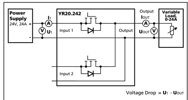
Fig. 18-3 Power losses when only one input is used
