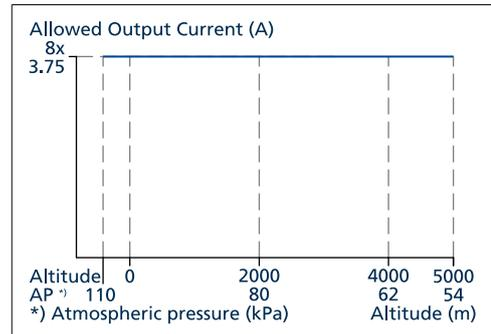
Fig. 18-2: Output current vs. altitude
