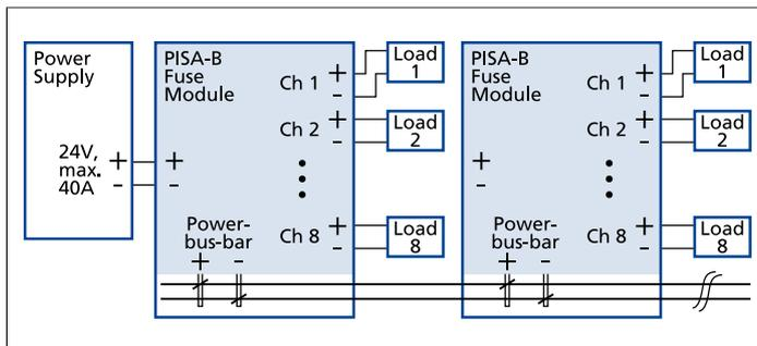
Fig. 3-3: Typical wiring scheme for multiple modules
