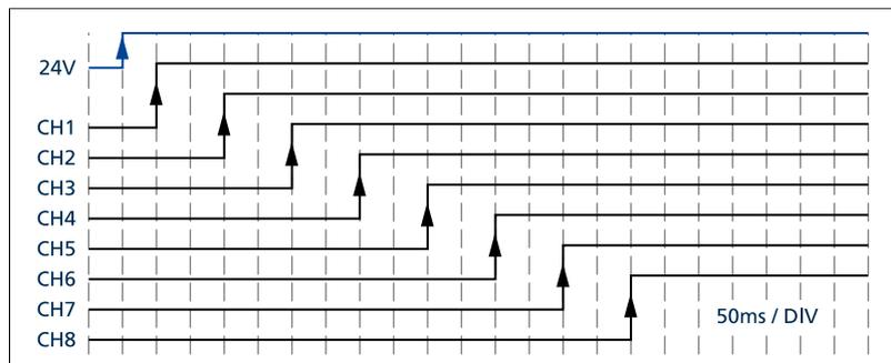
Fig. 5-1: Turn-On sequence after applying an input voltage
