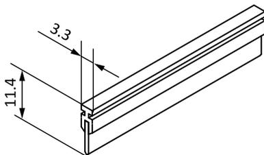
Fig. 23-1: Mechanical dimensions
