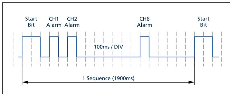
Fig. 8-1: Digital Coded Alarm Signal – Signal Sequence
