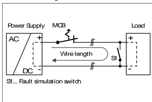
Maximal wire length<sup>\*)</sup> for a fast (magnetic) tripping:
