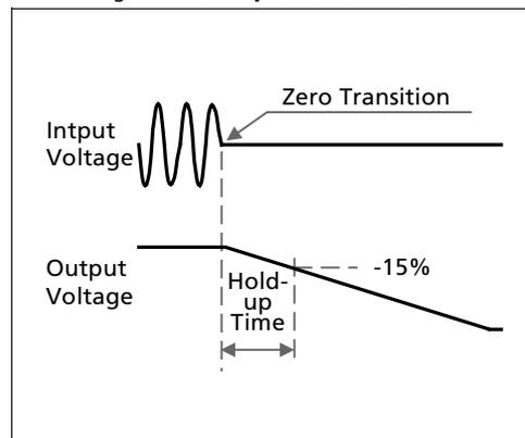
Fig. 8-2 Hold-up time vs. input voltage
