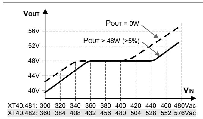
Fig. 5-2 **Input voltage range**
