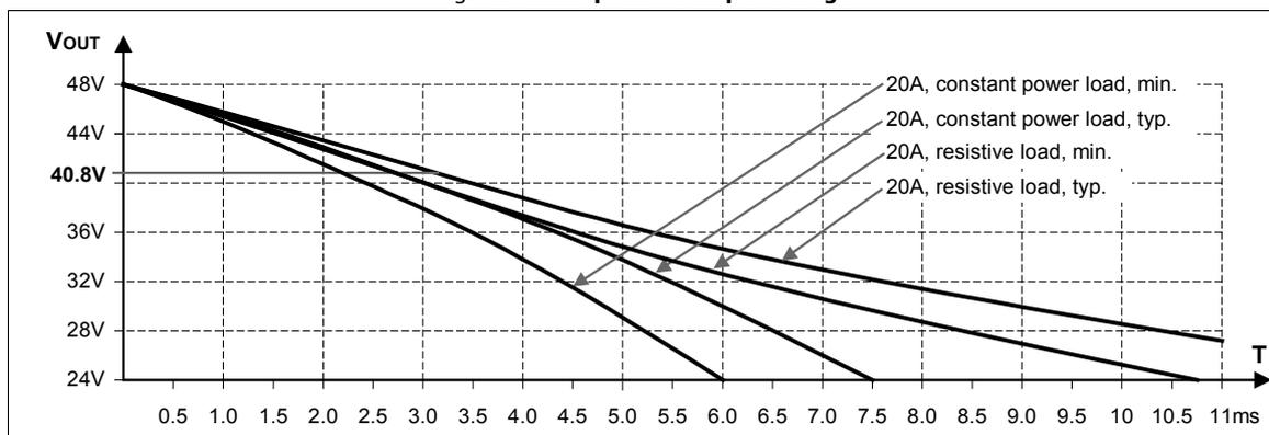
Note: At no load, the hold-up time can be up to one minute. The green DC-ok LED is on during this time.
