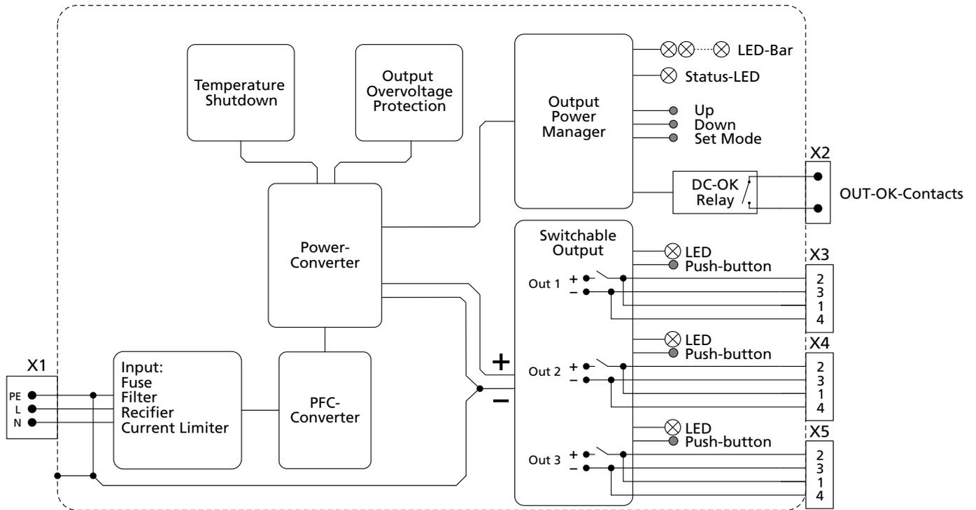
Fig. 12-1: Functional Diagram FPS300.245-049-102
