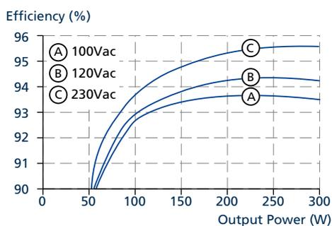
Fig. 9-1: Efficiency vs. output power at 24 V, typ.
