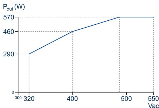
Fig. 23-1: Two phase power capability
