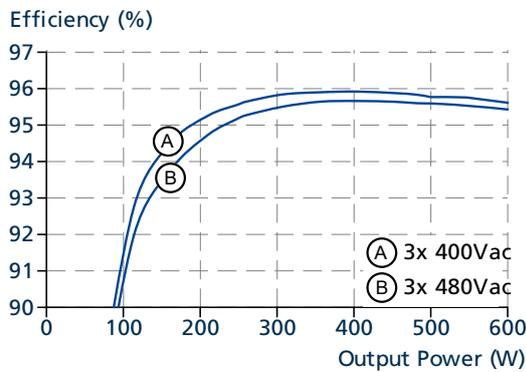
Fig. 9-1: Efficiency vs. output power at 24 V, typ.
