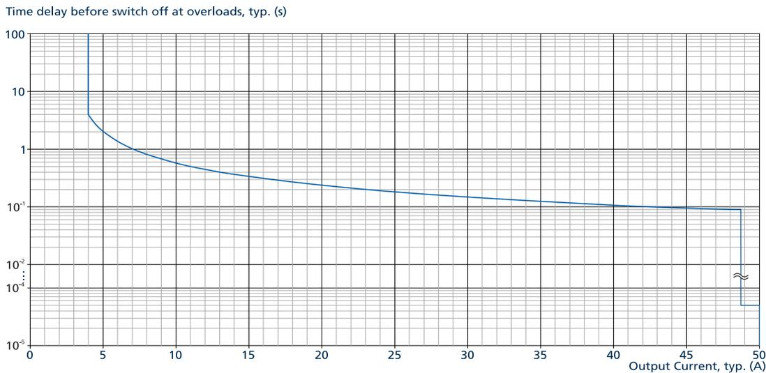
Fig. 6-4: Trip curve diagram for NEC Class II
