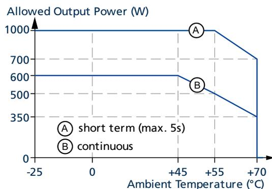
Fig. 16-1: Output power vs. ambient temp.
