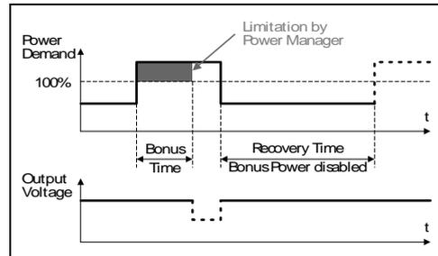
The BonusPower is available as soon as power comes on and immediately after the end of an output short circuit or output overload.
