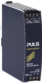
The YR40.242 is equipped with two input channels, which are individually decoupled by utilizing mosfet technology. Using mosfets instead of diodes reduces the heat generation and the voltage drop between input and output. The YR40.242 does not require an additional auxiliary voltage and is self-powered even in case of a short circuit across the output.
