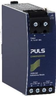
The YR80.242 is the preferred redundancy module for the CPS20.121 power supply. It is equipped with two input channels, which are individually decoupled by utilizing mosfet technology. Using mosfets instead of diodes reduces the heat generation and the voltage drop between input and output. The YR80.242 does not require an additional auxiliary voltage and is self-powered even in case of a short circuit across the output.
