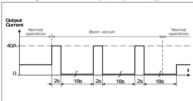
Fig. 6-4 Dynamic overcurrent capability, typ.
