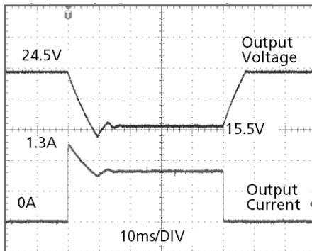
Peak load 1.3A (resistive load) for 50ms
