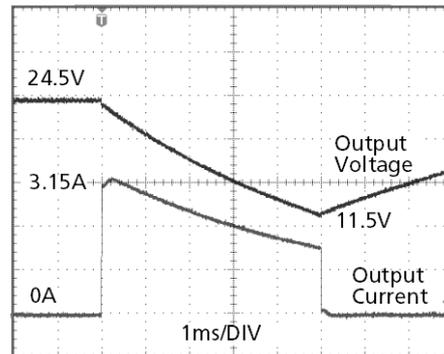
Peak load 3.15A (resistive load) for 5ms
