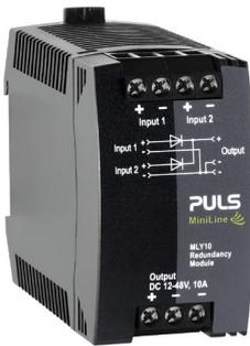
The MLY10.241 is a dual redundancy module, which has two diodes with a common cathode included. It can be used for various purposes. The most popular application is to configure highly reliable and true redundant power supply systems. Another interesting application is the separation of sensitive loads from non-sensitive loads. This avoids the distortion of the power quality for the sensitive loads which can cause controller failures.
