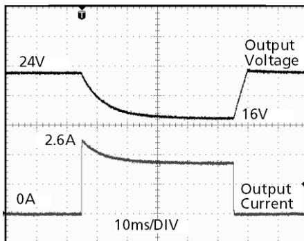
Peak load 2.6A (resistive load) for 50ms
