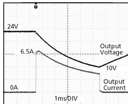
Peak load 6.5A (resistive load) for 5ms
