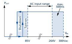
Fig. 3-1: Input voltage range
