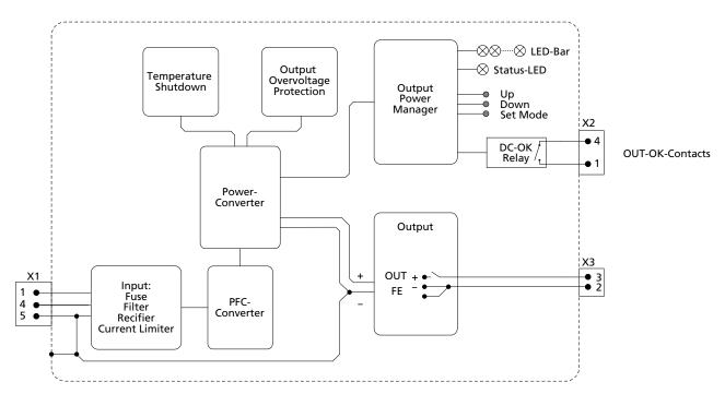
Fig. 12-1: Functional Diagram FPS300.241-002-101
