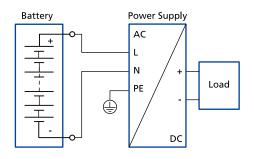
Fig. 4-1: Wiring for DC Input
