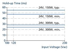
Fig. 7-1: Hold-up time vs. input voltage
