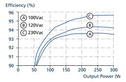
Fig. 9-1: Efficiency vs. output power at 24 V, typ.
