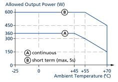
Fig. 16-1: Output power vs. ambient temp.
