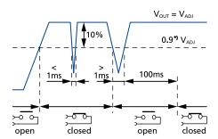
Fig. 8-1: DC-OK relay contact behavior
