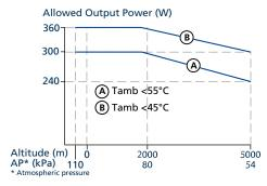
Fig. 16-2: Output power vs. altitude
