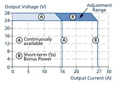
Fig. 6-1: Output voltage vs. output current
