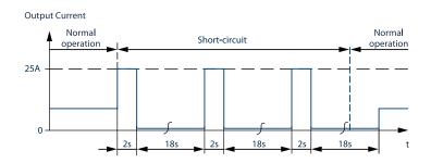
Fig. 6-2: Short-circuit on output, overcurrent mode, typ.
