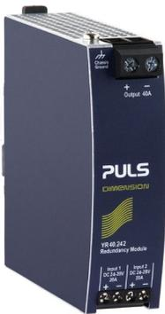
The YR40.242 redundancy module is equipped with two input channels, which are individually decoupled by utilizing MOSFET technology. Using MOSFETs instead of diodes reduces the heat generation and the voltage drop between input and output.
