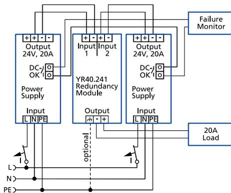
Fig. 24-5: 1+1 Redundant configuration for 20A load current with a dual redundancy module
