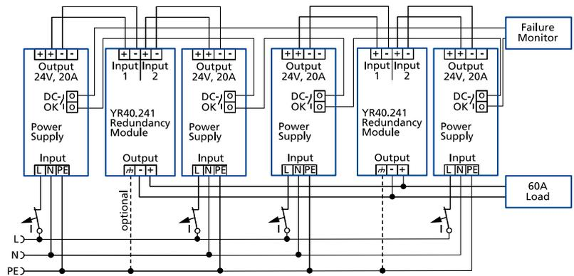
Fig. 24-6: N+1 Redundant configuration for 60A load current with multiple devices and redundancy modules
