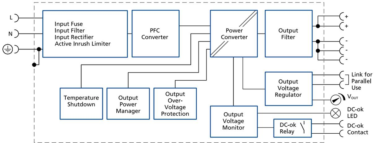
Fig. 12-1: Functional diagram
