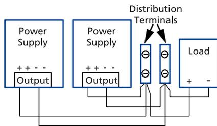
Fig. 13-1: Using distribution terminals
