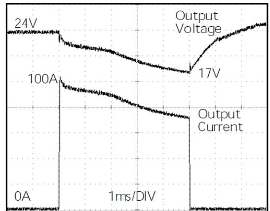
Fig. 24-2: 100A peak current for 5ms, typ. (5x the nominal current)
