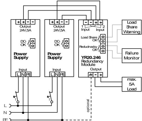
Fig. 23-6 N+1 Redundant configuration for 15A load current with multiple power supplies and redundancy modules
