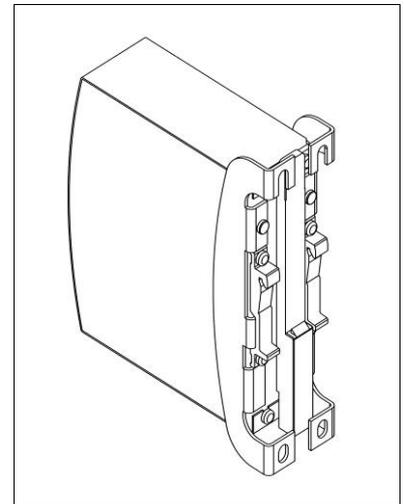
Fig. 22-4 Wall/panel mounting, front view
