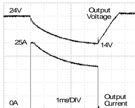
Fig. 23-3 15A<sub>peak</sub> current for 12ms, typ.
