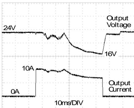
Fig. 23-2 25A<sub>peak</sub> current for 5ms, typ.
