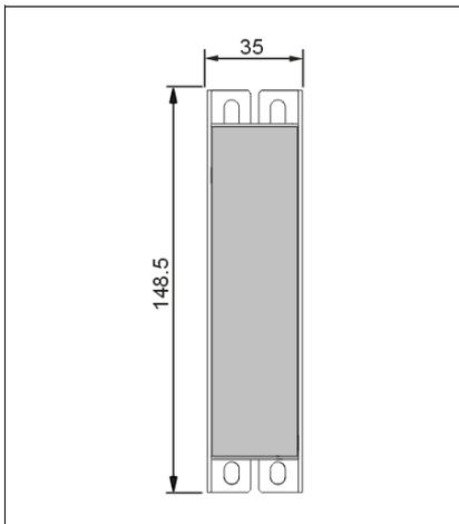
Fig. 22-5 Hole pattern for wall mounting
