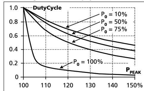
$$\text{DutyCycle} = \frac{T_{\text{peak}}}{T_{\text{peak}} + T_0}$$
