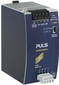
This buffer unit is a supplementary device for DC 24V power supplies. It delivers power to bridge typical mains failures or extends the hold-up time after turn-off of the AC power. In times when the power supply provides sufficient voltages, the buffer unit stores energy in integrated electrolytic capacitors. In case of mains voltage fault, this energy is released again in a regulated process. One buffer module can deliver 20A additional current.
