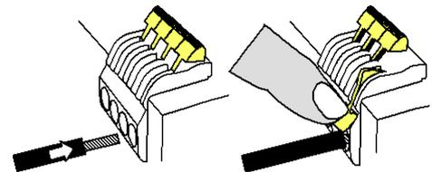
1. Insert the wire    2. Snap the lever
