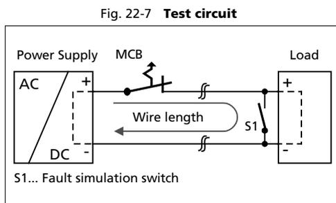
Maximal wire length<sup>\*)</sup> for a fast (magnetic) tripping:
