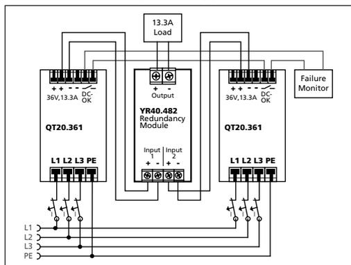
Fig. 21-7 Typical N+1 Redundant configuration for 40A with two dual redundancy modules and four power supplies
