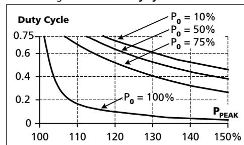
$$\text{DutyCycle} = \frac{T_{\text{peak}}}{T_{\text{peak}} + T_0}$$
