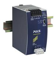
This buffer unit is a supplementary device for DC 48V power supplies. It delivers power to bridge typical mains failures or extends the hold-up time after turn-off of the AC power. In times when the power supply provides sufficient voltages, the buffer unit stores energy in integrated electrolytic capacitors. In case of mains voltage fault, this energy is released again in a regulated process.
