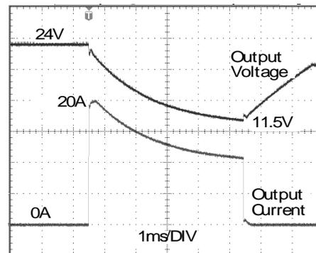
Peak load 20A (resistive load) for 5ms
