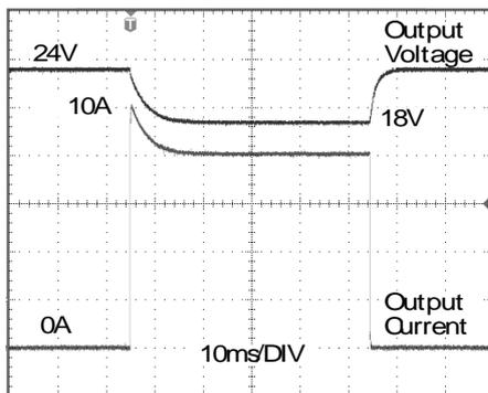
Peak load 10A (resistive load) for 50ms
