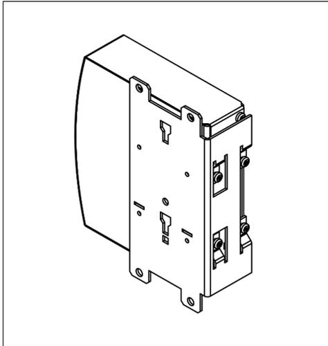
Fig. 23-6 Side mounting with DIN rail brackets\*)
