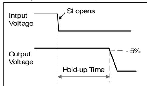
Note: At no load, the hold-up time can be up to several seconds. The green DC-OK LED is also on during this time.
