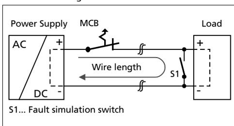
Maximal wire length<sup>\*)</sup> for a fast (magnetic) tripping:
