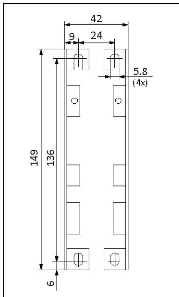
Fig. 23-6 Wall/panel mounting, side view
