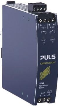
The YR2.DIODE is a dual redundancy module, which has two diodes as decoupling devices included. It can be used for various purposes. The most popular application is to configure highly reliable and true redundant power supply systems. Another interesting application is the separation of sensitive loads from non-sensitive loads. This avoids the distortion of the power quality for the sensitive loads which can cause controller failures.
