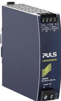
The YR40.482 is equipped with two input channels, which are individually decoupled by utilizing MOSFET technology. Using MOSFETs instead of diodes reduces the heat generation and the voltage drop between input and output. The YR40.482 does not require an additional auxiliary voltage and is self-powered even in case of a short circuit across the output.
