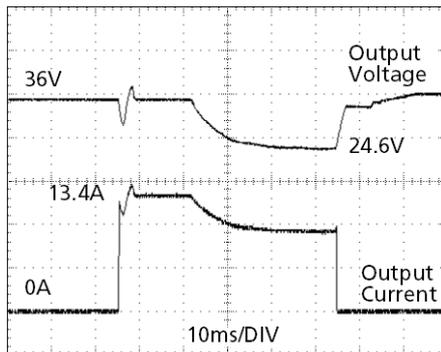
Fig. 24-2 **33.5A peak current for 5ms , typ. (5x the nominal current)**
