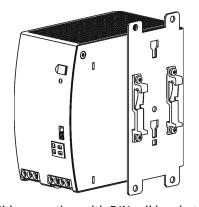
Side mounting with DIN rail brackets
