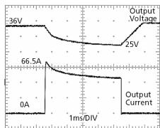
66.5A Peak load (resistive) for 5ms Output voltage dips from 36V to 25V.
