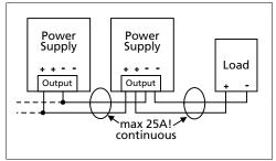
Fig. 12-2 Using distribution terminals
