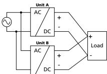
If more than three units are connected in parallel, a fuse or circuit breaker
