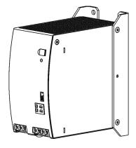
Due to the small size of the unit, it is required that the black-DIN rail slide on the back of the unit must be removed. Instructions how to do this can be found in the manual of the ZM2.WALL.
