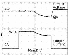
26.6A Peak load (resistive) for 50ms Output voltage dips from 36V to 26V.
