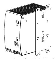
Side mounting without DIN rail brackets
