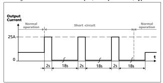
Fig. 6-4 Dynamic overcurrent capability, typ.
