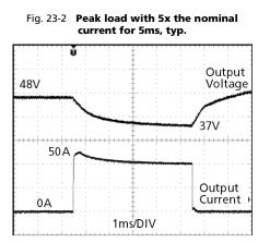
Peak load 50A (resistive) for 5ms Output voltage dips from 48V to 37V.
