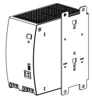
Side mounting without DIN rail brackets
