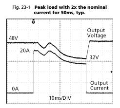
Peak load 20A (resistive) for 50ms Output voltage dips from 48V to 32V.
