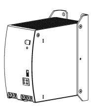
Due to the small size of the unit, it is required that the black-DIN rail slide on the back of the unit must be removed. Instructions how to do this can be found in the manual of the ZM2.WALL.
