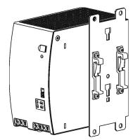
Side mounting with DIN rail brackets
