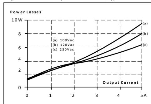
Fig. 8-3 Efficiency vs. input voltage at 24V, 5A, typ.
