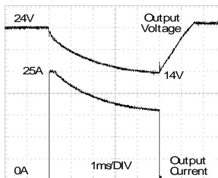
Fig. 23-3 15A peak current for 12ms , typ.
