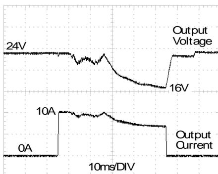
Fig. 23-2 25A peak current for 5ms , typ.
