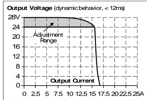
Fig. 5-3 Short-circuit on output, Hiccup<sup>PLUS</sup> mode, typ.
