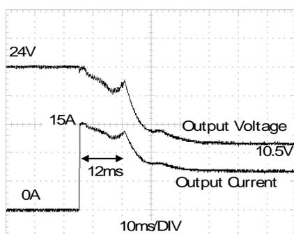
Please note: The DC-ok relay triggers when the voltage dips more than 10% for longer than 1ms.
