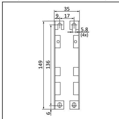
Fig. 22-6 Wall/panel mounting,
