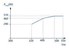
Fig. 22-1: Two phase power capability
