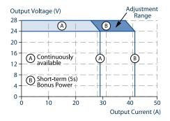
Fig. 6-1: Output voltage vs. output current
