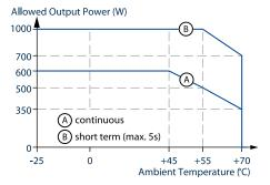
Fig. 16-1: Output power vs. ambient temp.
