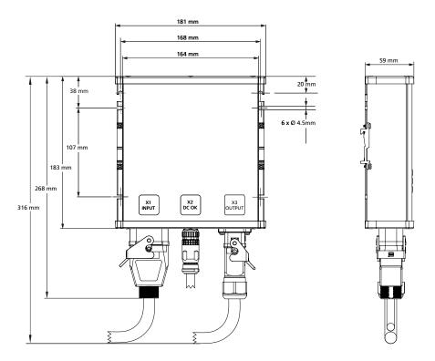
Width: 181 mm Height: 183 mm Depth: 59 mm Weight: 1200 g Housing body material: Housing cover material: Installation clearances:
