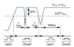
Fig. 8-1: DC-OK relay contact behavior
