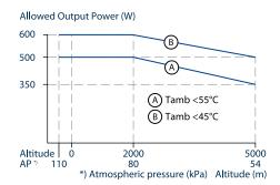
Fig. 16-2: Output power vs. altitude
