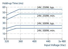
Fig. 7-1: Hold-up time vs. input voltage
