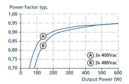
Fig. 3-4: Power factor vs. output power at 24 V output voltage
