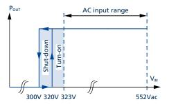
Fig. 3-1: Input voltage range
