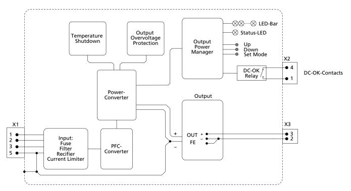
Fig. 12-1: Functional Diagram FPT500.241-002-101
