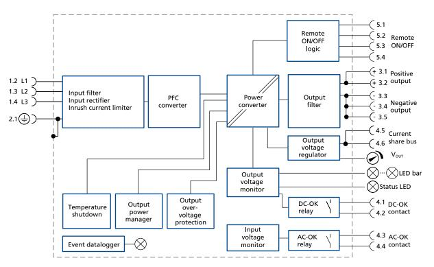
Fig. 17-1: Functional Diagram TP960.484
