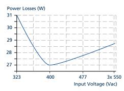
Fig. 14-4: Losses vs. input voltage at 48 V, 20 A, typ.
