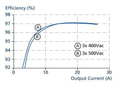
Fig. 14-1: Efficiency vs. output current at 48 V, typ.
