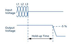
Fig. 8-2: Shut-down behaviour
