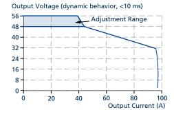
Fig. 7-2: Dynamic overcurrent capability, typ.
