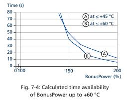
After operating at BonusPower, the power supply needs a cool-down period or recovery time. This can be calculated depending on the base load (<100 %) following the BonusPower period.
