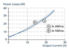
Fig. 14-2: Losses vs. output current at 48 V, typ.
