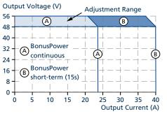
Fig. 7-1: Output voltage vs. output current, typ.
