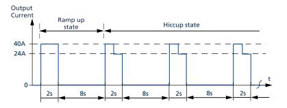
Fig. 7-3: Short-circuit on output, Hiccup<sup>PLUS</sup> mode, typ.
