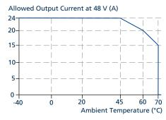
Fig. 22-1: Output current vs. ambient temp.
