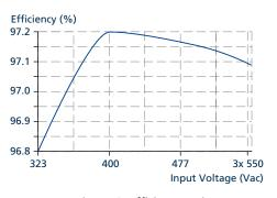
Fig. 14-3: Efficiency vs. input voltage at 48 V, 20 A, typ.
