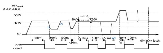
Fig. 10-1: AC OK relay contact behavior
