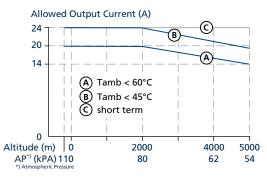
Fig. 22-2: Output current vs. altitude
