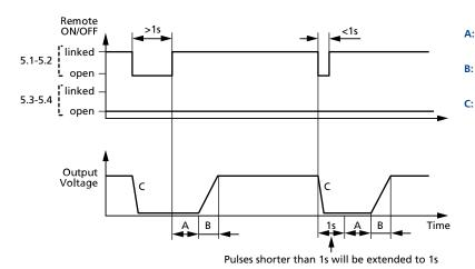
Turn-on delay according to Fig. 3-2: Turn-on behavior, definitions
