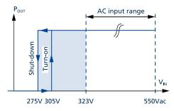
Fig. 3-1: Input voltage range
