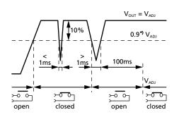
Fig. 9-1: DC OK relay contact behaviour
