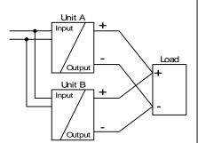
The output voltages of all DC/DC converters shall be adjusted to the same value (±100mV) at
