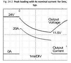
Peak load 20A (resistive load) for 5ms Output voltage dips from 24V to 11.5V.
