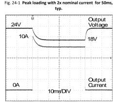
Peak load 10A (resistive load) for 50ms Output voltage dips from 24V to 18V.
