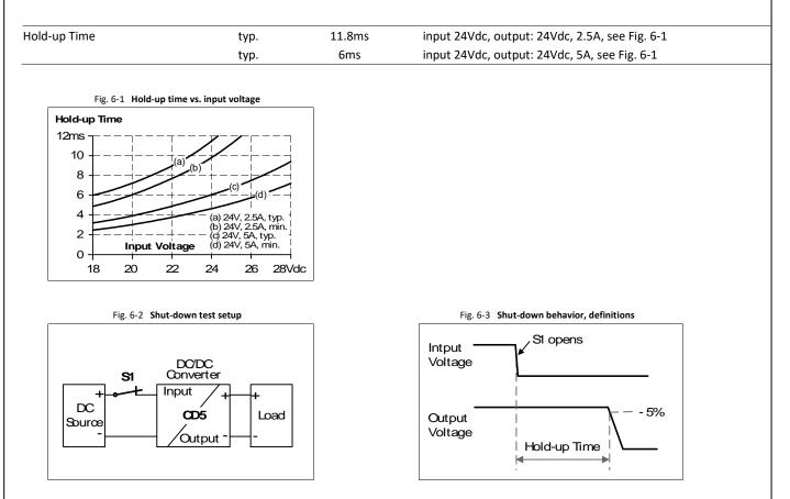
Note: At no load, the hold-up time can be up to several seconds. The green DC-OK LED is also on during this time.
