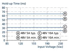
Fig. 7-1: Hold-up time vs. input voltage
