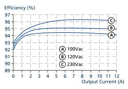
Fig. 9-1: Efficiency vs. output current at 48 V, typ.
