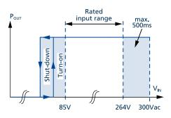
Fig. 3-1: Input voltage range
