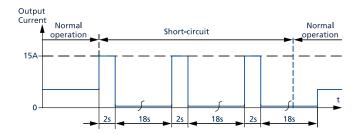
Fig. 6-3: Short-circuit on output, Hiccup<sup>PLUS</sup> mode, typ.
