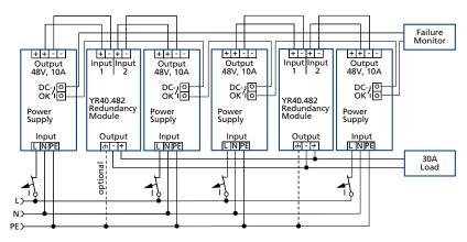
Fig. 24-6: N+1 Redundant configuration for 30A load current with multiple devices and redundancy modules
