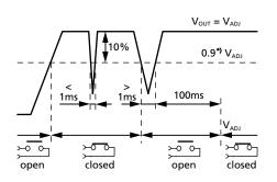
Fig. 8-1: DC-ok relay contact behavior
