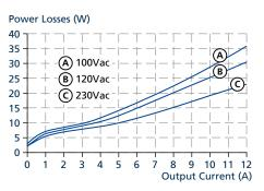
Fig. 9-2: Losses vs. output current at 48 V, typ.
