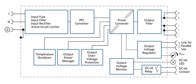
Fig. 12-1: Functional diagram
