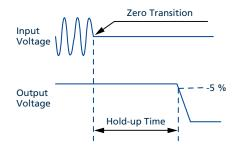
Fig. 7-2: Shut-down behaviour, definitions
