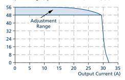
Fig. 6-2: Dynamic overcurrent capability, typ.
