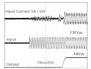
Fig. 5-1: Typical turn-on behaviour at nominal load and 25°C ambient
