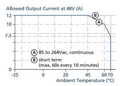
Fig. 16-1: Output current vs. ambient temp.  $(I_{nom} = 10A; I_{out} \text{ with PowerBoost} = 12A)$
