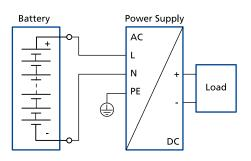
Fig. 4-1: Wiring for DC Input
