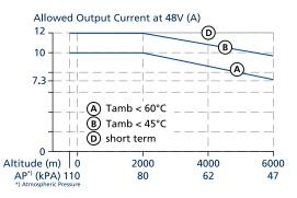
Fig. 16-2: Output current vs. altitude
