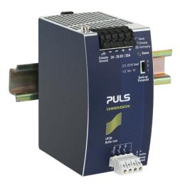
The UF20.481 buffer module is a supplementary device for DC 48V power supplies. It delivers power to bridge typical mains failures or extends the hold-up time after the AC power is turned off.
