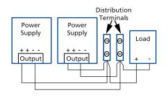
Fig. 13-2: Using distribution terminals
