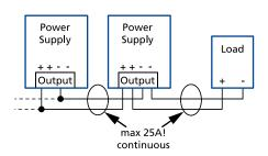
Fig. 13-1: Daisy chaining of outputs
