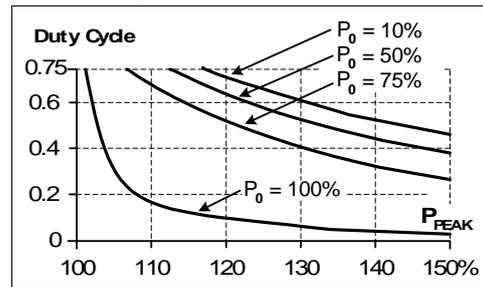
$$\text{DutyCycle} = \frac{T_{\text{peak}}}{T_{\text{peak}} + T_0}$$
