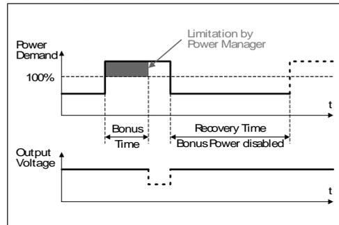
The BonusPower is available as soon as power comes on and after the end of an output short circuit or output overload.
