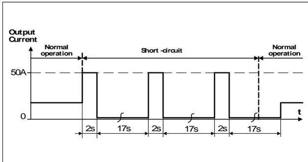
Fig. 6-4 Dynamic overcurrent capability, typ.
