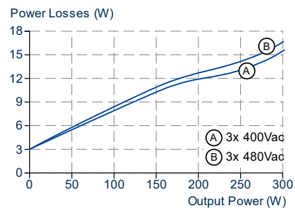
Fig. 9-2: Losses vs. output power at 24V, typ.
