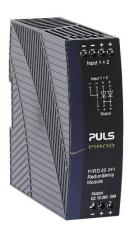
The PIRD20.241 is a very cost effective diode redundancy module, which can be used to build 1+1 and N+1 redundant systems. It is equipped with two input channels, which can be connected to power supplies with up to 10A output current and one output, which can carry nominal currents up to 20A.
