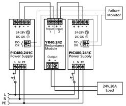
d) It is desirable to set the output voltages of all units to the same value (± 100mV) or leave it at the factory setting.
