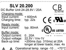
Operational temp. range -10 ... +70°C Do not open, risk of electrical shock Label-Nr. 346.920.00X www.puls-power.com Made in Czech Republic
