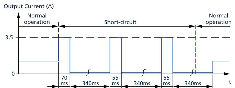
Fig. 6-2: Intermittent current at short circuit, typ.\*)
