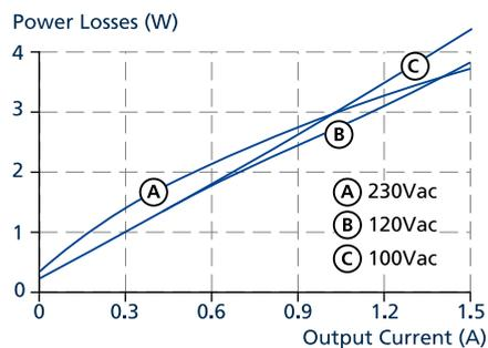
Fig. 8-2: Losses vs. output current at 24V, typ.
