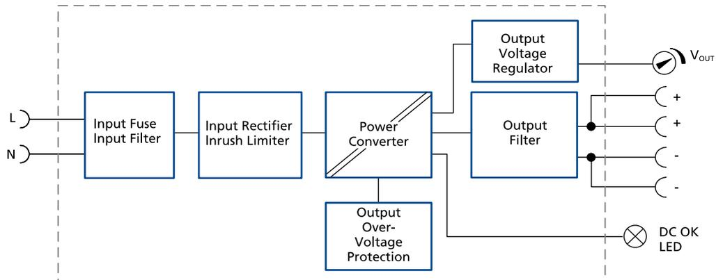
Fig. 11-1: Functional diagram
