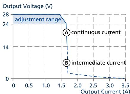
Fig. 6-1: Output voltage vs. output current, typ.
