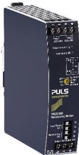
The YR20.246 is equipped with two input channels, which are individually decoupled by utilizing MOSFET technology. Using MOSFETs instead of diodes reduces the heat generation and the voltage drop between input and output. The YR20.246 does not require an additional auxiliary voltage and is self-powered even in case of a short circuit across the output.
