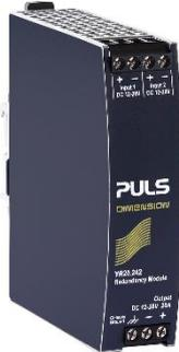
The YR20.242 is equipped with two input channels, which are individually decoupled by utilizing MOSFET technology. Using MOSFETs instead of diodes reduces the heat generation and the voltage drop between input and output. The YR20.242 does not require an additional auxiliary voltage and is self-powered even in case of a short circuit across the output.
