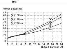
Fig. 11-4 Losses vs. input voltage at 24 V, 20
