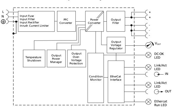
Fig. 12-1 Functional diagram
