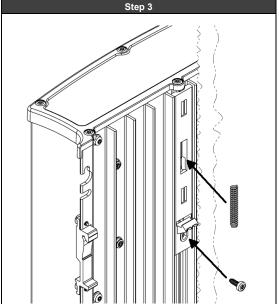
Put the spring over the plastic guide pin, compress it and push it into the grove. Fix the slider with the screw. Use a torque of 0.8Nm/7.08 lbf inch
