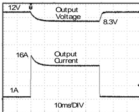
Peak load 16A (resistive load) for 50ms
