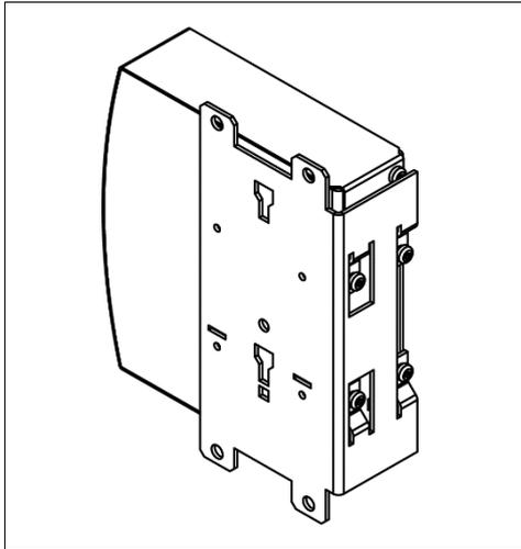
Fig. 21-6 Side mounting with DIN rail brackets\*)
