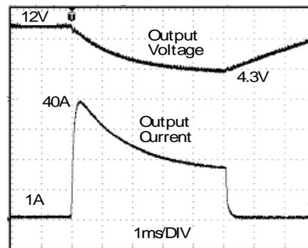
Peak load 40A (resistive load) for 5ms
