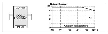
Fig. 22-7 Mounting Orientation B (Upside down)
