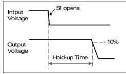
Note: At no load, the hold-up time can be up to several seconds. The green DC-OK LED is also on during this time.
