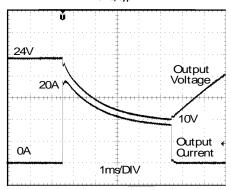
Peak load 20A (resistive load) for 5ms Output voltage dips from 24V to 10V.
