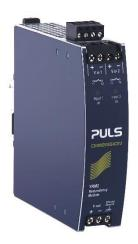
The YRM2.DIODE is a dual redundancy module, which can be used to build 1+1 and N+1 redundant systems. It is equipped with two input channels, which are individually decoupled by utilizing diodes.
