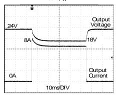
Peak load 8A (resistive load) for 50ms Output voltage dips from 24V to 18V.
