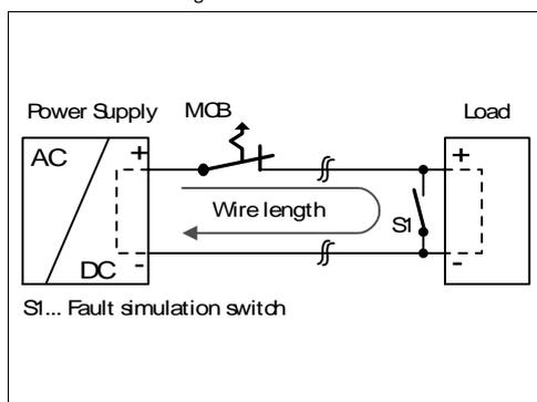
Maximal wire length<sup>1)</sup> for a fast (magnetic) tripping:
