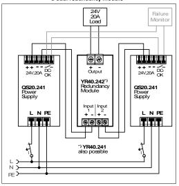
Fig. 22-2 Typical N+1 or 1+1 Redundant configuration for 20A with multiple YR40.245 redundancy modules
