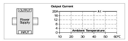
Fig. 23-7 Mounting Orientation B (Upside down)
