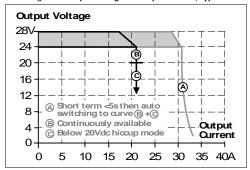
Fig. 6-3 Short-circuit on output, hiccup mode (typ.)
