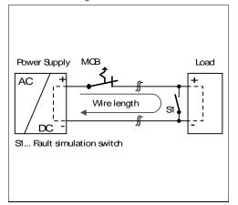
Maximal wire length\*) for a fast (magnetic) tripping:
