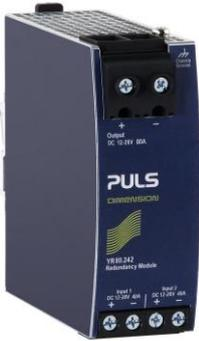
The YR80.242 is equipped with two input channels (40A each), which are individually decoupled by utilizing mosfet technology. The output current can go as high as 80A. Using mosfets instead of diodes reduces the heat generation and the voltage drop between input and output. The YR80.242 does not require an additional auxiliary voltage and is self-powered even in case of a short circuit across the output.
