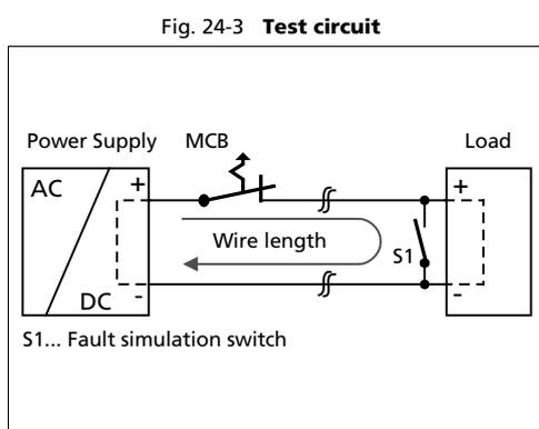
Maximal wire length\*) for a fast (magnetic) tripping:
